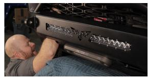
15. Install the small brackets that connect the factory bumper ends to the new bumper. Loosely install the hardware then pull the factory bumper end toward the new bumper and tighten the bolts. This will allow you to adjust the gap between the Blitz bumper and the factory plastic.
