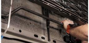
14. Mount the bumper. Have a friend help you or use a jack. Once you get the bumper mounted on the frame, loosely tigthen the two inside bolts first, then tighten the three outside bolts on both sides. After you get all of the bolts loosely installed, tighten them down.
