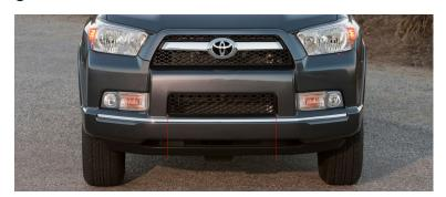
**9.** Use a 10mm socket and remove the 2 bolts on the bottom skid. Remove the bolts connecting the inner fender to the bumper bracket.
