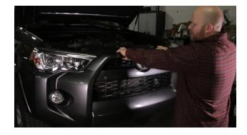
5. Remove the bumper. Gentley pull the bumper away from the vehicle to release the snaps. Make sure not to pull the bumper completely off because the fog lights are still connected. Once you get 1 side loose, disconnect the fog lights so you can remove the entire bumper.
