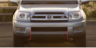
If you are installing a 5th gen (10-13) Blitz. You will cut along the red lines below and remove the center portion of the factory bumper/lower plastic grill. The rest of the install will be the same.
