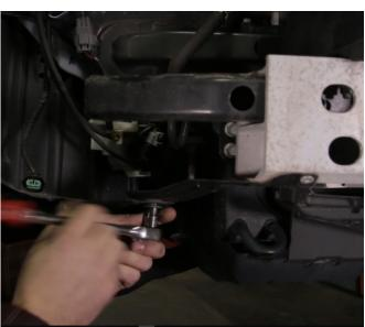
10. Use a 14mm socket and remove the bumper mounting bolts. There are 3 on the outsid eof the frame rail and 1 on the inside of the frame rail. Repeat the same steps on the other side. Remove the factory bumper and then reinstall the factory plastic cover we removed earlier.
