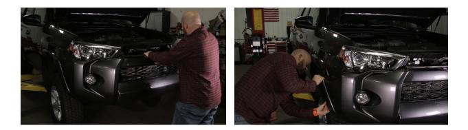
**6.** Place tape inside the curve of the bumper as shown in the picture below to make our cut line and to protect the paint. We will also be cutting the front face of the bumper so tape a line 3/8" down from the grill.
