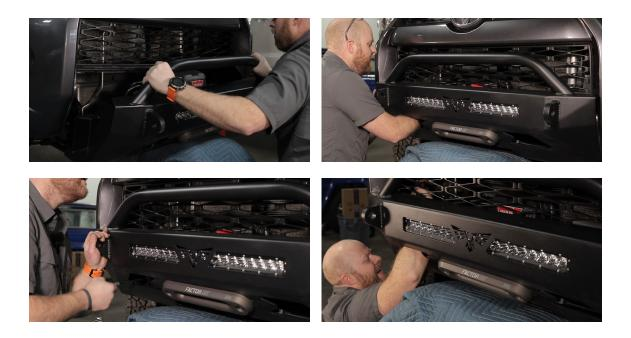
**15.** Install the small brackets that connect the factory bumper ends to the new bumper. Loosely install the hardware then pull the factory bumper end toward the new bumper and tighten the bolts. This will allow you to adjust the gap between the Blitz bumper and the factory plastic.
