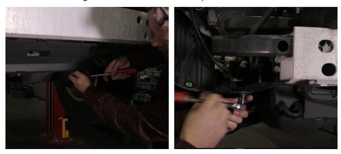
**10.** Use a 14mm socket and remove the bumper mounting bolts. There are 3 on the outsid eof the frame rail and 1 on the inside of the frame rail. Repeat the same steps on the other side. Remove the factory bumper and then reinstall the factory plastic cover we removed earlier.
