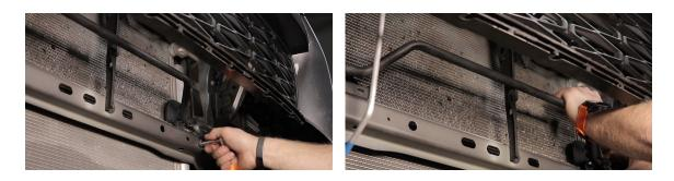
14. Mount the bumper. Have a friend help you or use a jack. Once you get the bumper mounted on the frame, loosely tigthen the two inside bolts first, then tighten the three outside bolts on both sides. After you get all of the bolts loosely installed, tighten them down.
