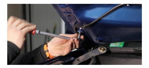
2. Once the bolts are removed, take the supplied bracket and line the bolt holes on the hinge up with the vertical slot on the bracket and loosely thread the factory bolts back into the hood to secure the bracket. You may need to adjust the depth of where the bracket sits so it doesn't hit the windshield when you close the hood. You can carefully and slowly close your hood to verify, once you have the distance set, fully tighten down the bolts with a 12mm socket.
