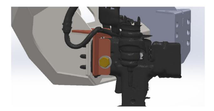
**10.** Next, put the supplied bolts through the top of the tie-in brackets and the bumper to locate the bracket on the frame. Once located, drill a 5/8" hole through the side of the bracket and the frame rail. Be sure to touch up any exposed metal with paint.
