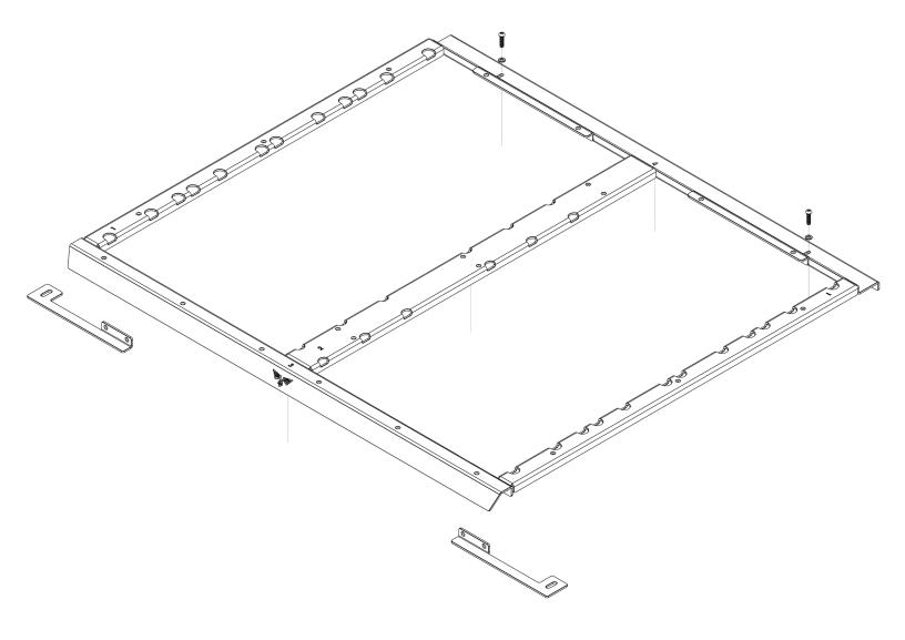
**10.** Next you will need to install the nut strip brackets in the front of the cargo space to the frame. To do so, take (2) of the provided button heads and washers and thread them through the back of the slots in the frame to the pems in the brackets, as shown in the orientation below. Be sure to do this process on both sides.
