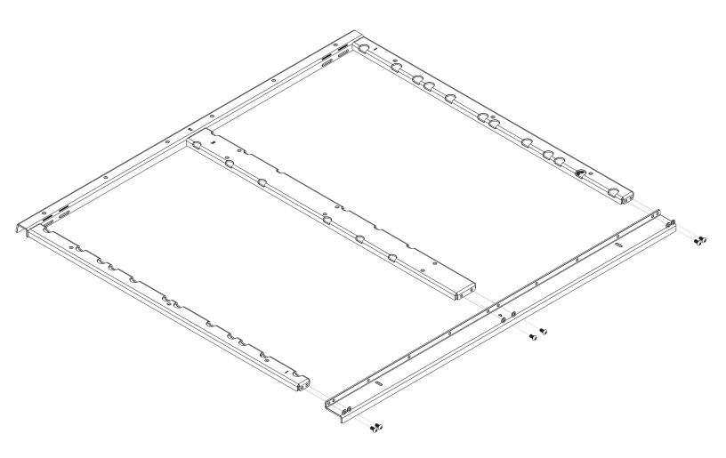
**4.** Now that the skeleton of the floor is assembled and tight, you now need to install the (2) provided support brackets with the 2 pems in them that the floor will bolt into. To do so, take the provided 1/4" button heads, washers and flange nuts and install them in the orientation shown below. Be sure to have the flanges with the pems in them facing up.
