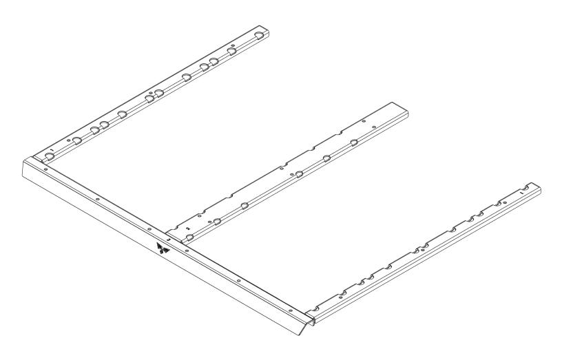
**3.** With all (3) brackets now assembled and tight, you can install the provided back bracket using the 1/4" button heads, washers and flange nuts. Be sure to install in the orientation below with the back flange down.
