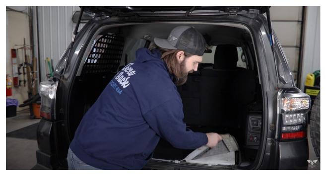
7. With the corner peeled back, take a razor blade or box cuter and use it to cut and trim back the thin plastic flange under the edge where you removed the hook assembly from. With this done you are able to slide our bracket under the plastic to fasten to the bolt hole where the hook was secured. One you have made that modification, you can fold and clip the corner back down to how it was, and also place and clip the rear plastic trim piece back down that was removed.
