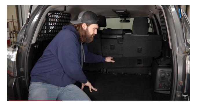
6. You now need to remove the rear plastic trim section on the floor, to do so use a plastic pry tool or a flathead screw driver to get under the plastic to pop it up. Once the plastic is popped up enough to get your fingers under it, you need to pull straight up to free up all the clips before you can remove the piece as a whole. Once the piece is removed, pull up the passenger side corner using your pry tool, as shown below.
